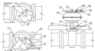
The unit now is properly armed and may be operated closed-open in the normal manner using valve handle (#5)
